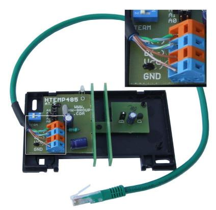
There is an older version of sensor on the picture but the cable connection is the same.
