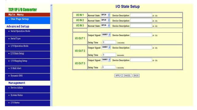
The ATC-2000 I/O offers a very smart and easy method to operate I/O function. You do not need to own any programming background. All you need to do is just making the relationship rules with each I/O. For example, if
