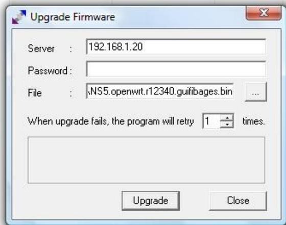
7. Signal LEDs will keep blinking one by one in 4 different colors during firmware upgrade. Wait for about 7-10 minutes (devices and firmware depending) - do not power off the device during the procedure!
