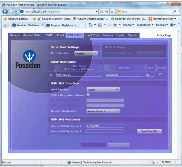
In the default setting you just need to set the remote IP of the Poseidon and the SMS phone numbers. The **SMS+ Ring when Alarm** is optional.
