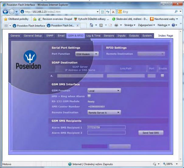
In the default status you first need to enable the GSM modem in the *Serial port Settings* and then set the *GSM Function* to *Local*. Deactivating the *SOAP destination* is optional, as well as the *SMS+ Ring when Alarm* function.
