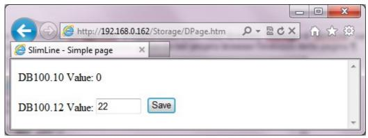
As can be seen, the top row shows the value of the PLC DB100.10 while setting a value in the text box in the bottom row and then pressing the *Save* button, you can set the value of the DB100.12.
