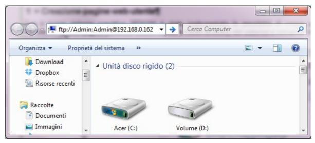
Here's the view of the file system at the connection. **Project** and **System** folders are reserved for system use and you should not change its contents. The files of the user pages can be transferred in the **Storage** and **SDCard** (if present) folders.
